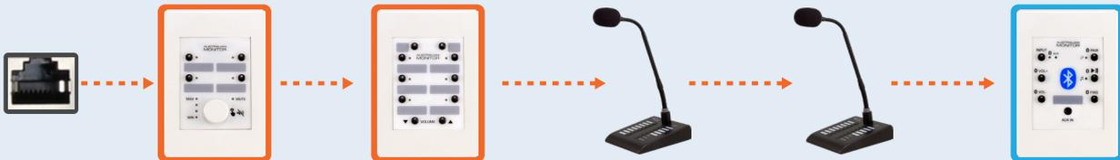
**!** Please note that accessory port local audio input channels are locked to the corresponding output zone and only one can be used per zone. E.g. Accessory port 1 local input connects to Zone 1. However, multiple wall panels and paging stations can be connected on the same accessory port.
