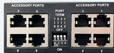
2. Terminate the LAST RS485 accessory on the port cable run.
