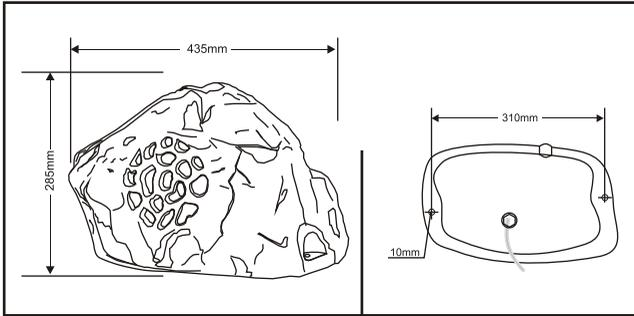
Thank you for choosing the Sonodyne RS 650i. In gardens and pool sides, where wall mounting speakers are not an option, and a minimalistic look is desired, the unique rock speaker, the RS 650i is a perfect fit. Moulded from FRP (Fibre Reinforced Plastic) the RS 650i enclosure resembles a rock and has a high grade 6" coaxial transducer with exceptional sound quality. It is 100% waterproof and has 100 V connectivity option
